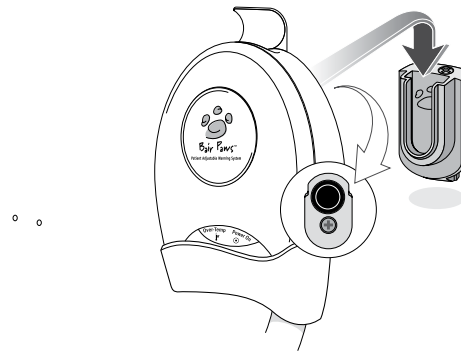
Figure 6. Mounting the warming unit with a suction wall mount adapter.
