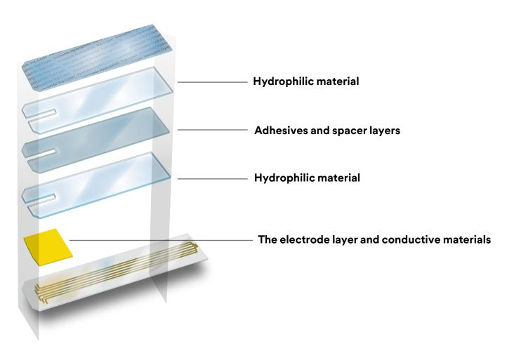
The layers working together ensure a repeatable sample is presented for analysis.
