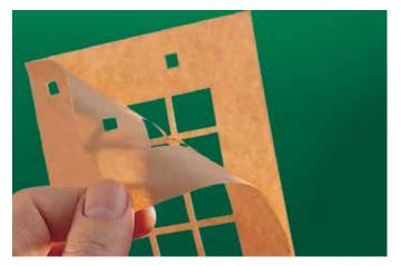
**Rotary die cutting:** Rotary die cutting is a common method in microfluidic device converting. This technique consists of using a precision patterned hard-tool of the desired shape to cut a film or substrate. The patterned tool is cylindrical and rotates in index with the moving web to cut a flat design. The benefits of using a rotary die over laser cutting are its increased line speed potential, lower cost of entry, and high degree of durability.
