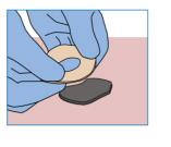
Fully insert the tube fitting into the tubing.
