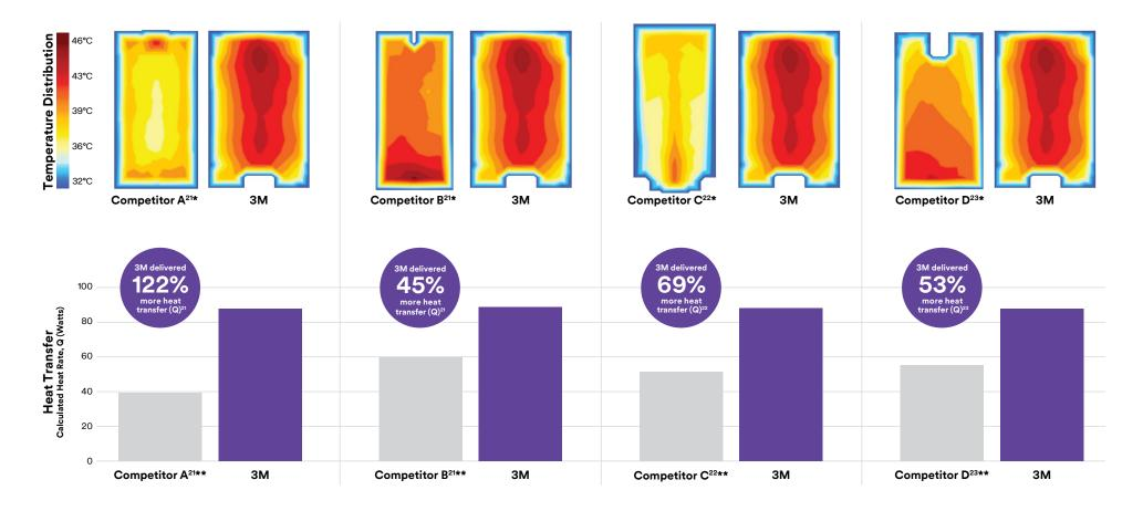
\*Images reflect the temperature of the portion of the blanket that transfers heat when inflated (tested per IEC 60601-2-35:2020), without showing additional brand identifying features. Competitive (full/lower/upper) body blanket used in conjunction with a full sized blower (120V/60hz) on its highest temperature and fan speed settings.
