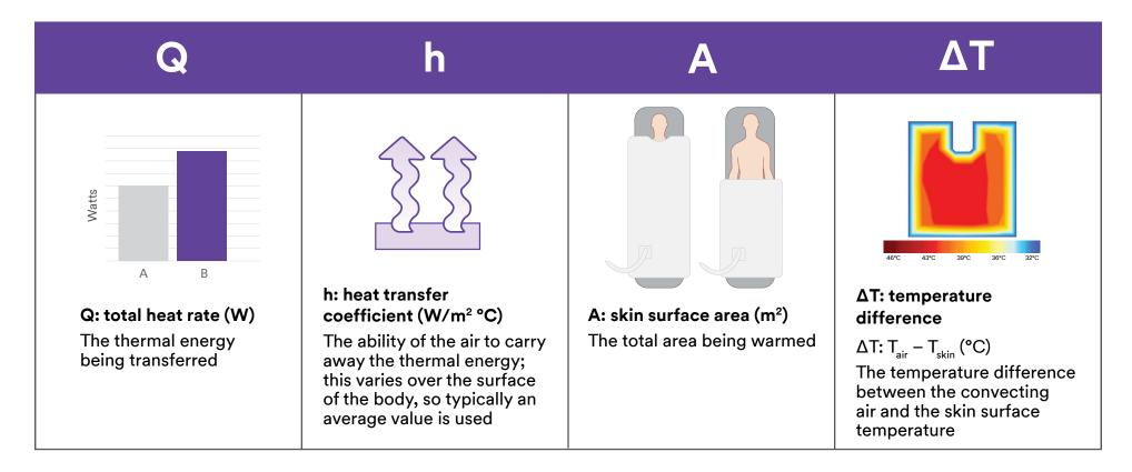
While the area (A) is typically very similar across forced air warming systems, the heat rate (Q), heat transfer coefficient (h) and temperature difference ( $\Delta$ T) can vary greatly and can have an impact on performance. These values were tested to determine what differences exist among various systems in comparison to the 3M<sup>™</sup> Bair Hugger<sup>™</sup> Warming System.
