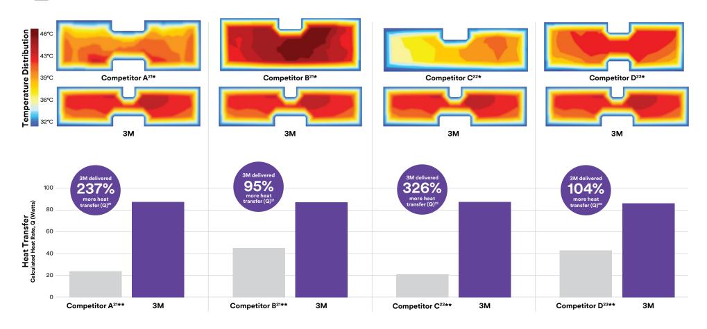
\*Images reflect the temperature of the portion of the blanket that transfers heat when inflated (tested per IEC 60601-2-35:2020), without showing additional brand identifying features. Competitive (full/lower/upper) body blanket used in conjunction with a full sized blower (120V/60hz) on its highest temperature and fan speed settings.
