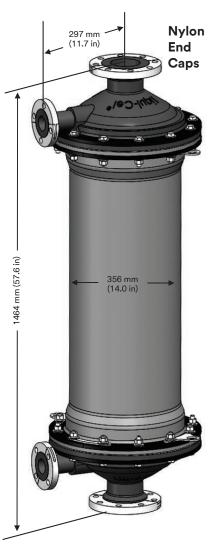
NOTE: Overall length with engineered thermoplastic end caps is 1466 mm (57.7 in). All dimensions are nominal values. See full housing drawings on 3M.com/Liqui-Cel for additional details.
