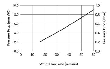
Test condition O₂ Removal: Vacuum mode with water at 35°C. Vacuum: 50 torr
