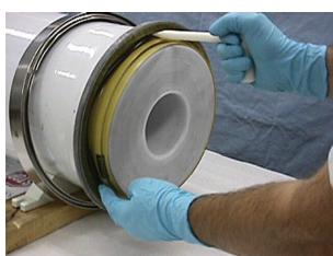
(G) Use the T-Handle insertion tool to press in the remaining O-ring sections. When inserting the O-rings, it is best to always divide each section of un-inserted O-ring in half and press in the middle section. See the photograph below, for an example.
