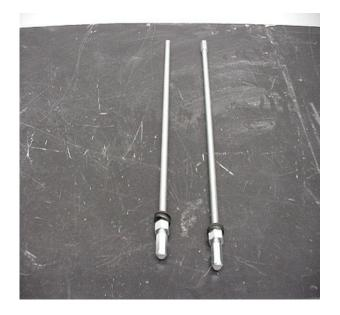
The end cap assembly tool is packaged and shipped unassembled. Upon receipt, assemble as shown. Typically, hand tightening the nuts is adequate.
