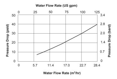
Curves represent nominal values with FRP housing using water at 20°C. Characteristics may change under different operating conditions.
