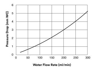
Test condition O₂ Removal: Vacuum mode with water at 25°C. Vacuum: 50 torr
