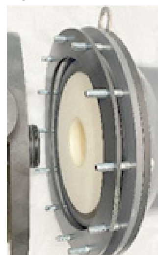
Figure 3: End cap moved away from the vessel
