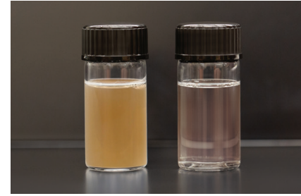
Before and after using 3M™ Harvest RC Chromatographic Clarifier: turbidity reduction in a single stage
